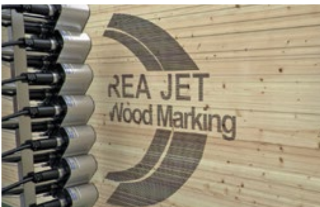
Large marking of logos on stacked boards
