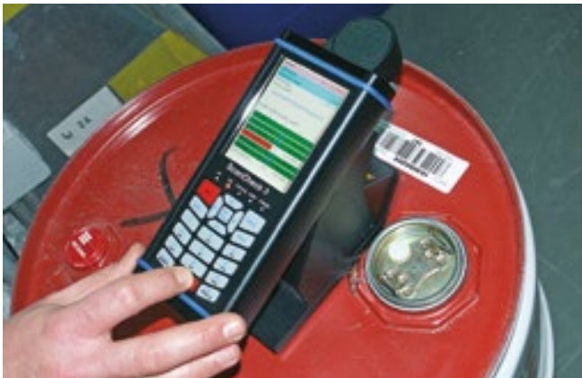
Verification of barcodes on metal drums
