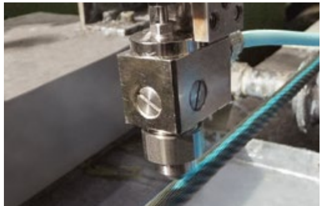
Color marking of wire cables
