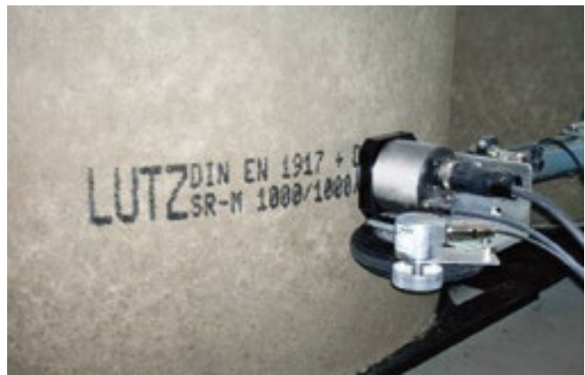
Marking of concrete pipes
