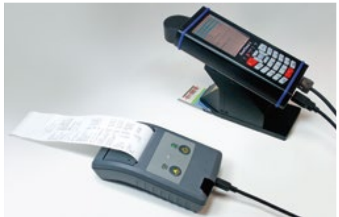
Creation of test reports on site
